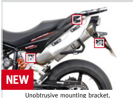
Unobtrusive mounting bracket.
